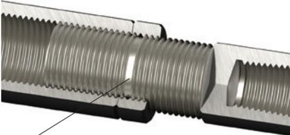
*Groove is completely hidden within locknut*
