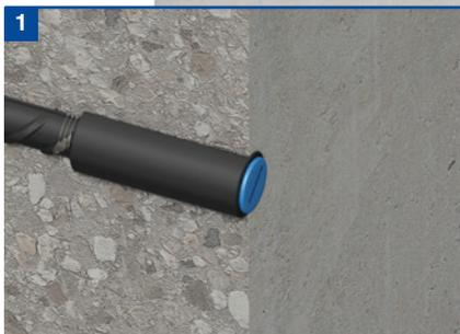
1 The coupler is normally supplied fixed to the reinforcing bar, ready to be installed and cast in concrete.
